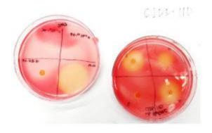
These Petris dishes are called a carboxymethylcellulose (CMC) plate assay, a test for activity of the enzymes. The clear areas indicate an active cellulase enzyme: The plate on the right in the image below shows that one of the genes that Matt's students is testing encodes a novel enzyme that can efficiently break down cellulose.
